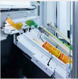
**2** After two pairs of channels are filled and the manipulator has arrived at the loading station, the hold-back flaps open and the two tracks of packages slide down simultaneously onto the two width-adjusted manipulator channels.
