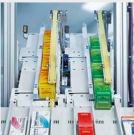
**4.1** If enough free capacity is available, the full track of packages can slide down at once, resulting in a very fast filling time. Stock levels in the final storage channels get identified by a laser sensor pointing into the respective channel.
