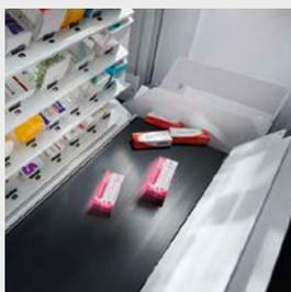
**4** Several medicine packages are collected in rapid succession, before being taken by the internal conveyor belt to a lift on one or both sides of the Consis H robot.
