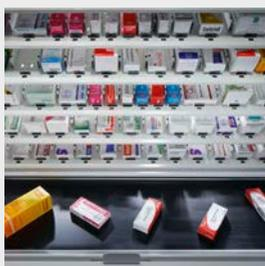
**3** Thanks to the intelligent CONSIS technology, the packages of a complete prescription, including 7 different items or more, can all hit the conveyor belt at virtually the same time.
