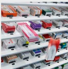
**2** Once ordered via your pharmacy software, packages drop from the channels onto an internal conveyor belt.
