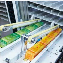
**4** Once positioned correctly, the manipulator can release the packages into the final storage channels by two different methods:
