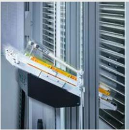
**3** After loading, the manipulator can run from the loading station to the final storage destinations at high speed, holding the packages safely with its side rails.
