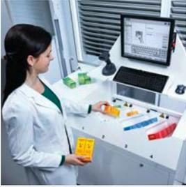
**1** Scanning and placing the packages in rows on the inclined channels of the loading station is easy. Because there are two pairs of channels, the user can constantly fill the device while the robot loads, alternating between the two pairs of channels.
