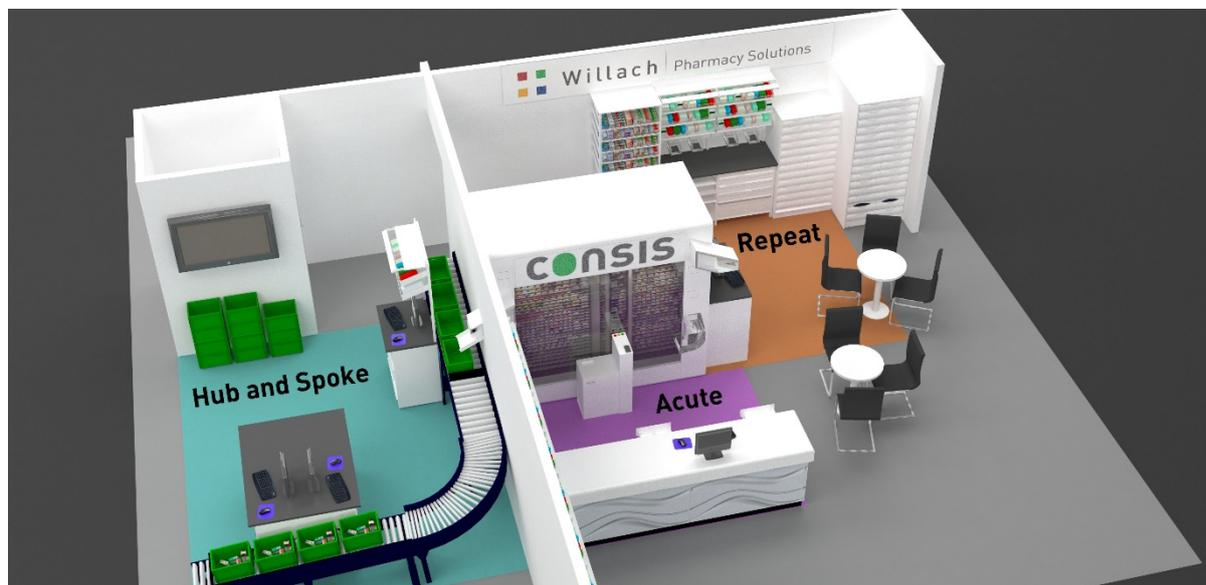
In a hub-and-spoke model, repeat prescriptions from one or many branches will be dispensed using a CONSIS robot in a centrally located pharmacy. The items for each repeat prescription are automatically labelled, dispensed and separated into containers. The prescriptions are then checked and packaged in bags. The already checked and bagged prescriptions are returned to the correct pharmacy daily. The bagged medication can then be stored in FAMA.M/comfort drawers awaiting collection.
